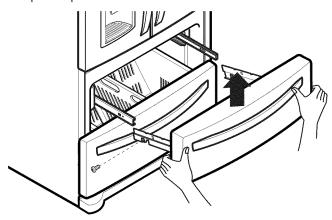
**4.** With both hands, flex the center bar enough to allow the gears on both ends to release from the track.
